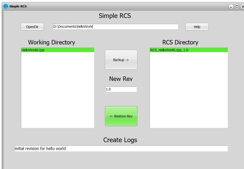
Figure 8: initiating a restore/revert from previous backup
